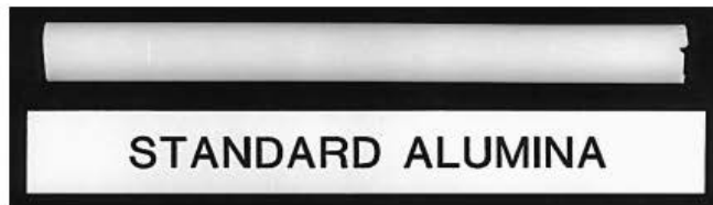
Figure 1-20 Porous microstructure in polycrystalline \text{Al}_2\text{O}_3 (a) leads to an opaque material (b). Nearly pore-free microstructure in polycrystalline \text{Al}_2\text{O}_3 (c) leads to a translucent material (d). (Courtesy of C. E. Scott, General Electric Company)
