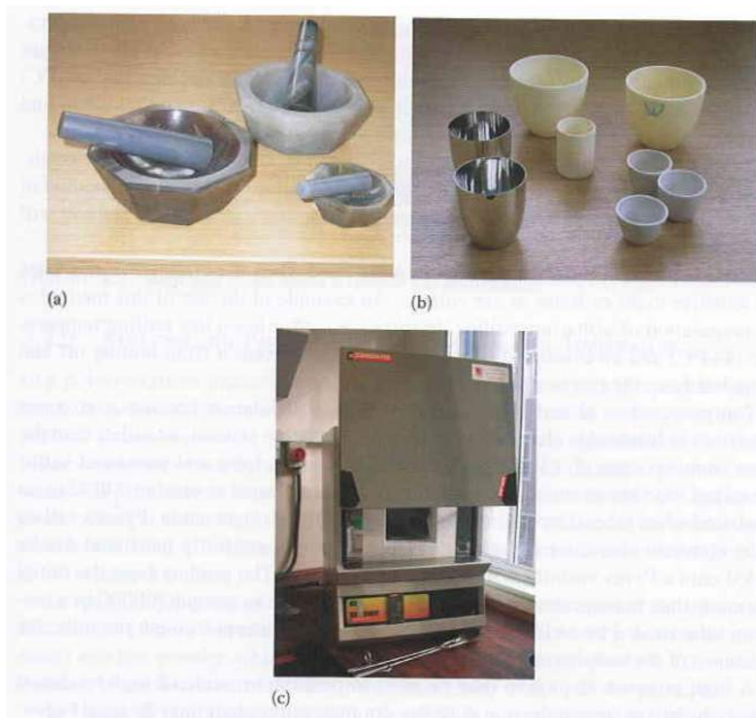
FIGURE 3.1 The basic apparatus for the ceramic method: (a) pestles and mortars for fine grinding; (b) a selection of porcelain, alumina and platinum crucibles; and (c) a furnace.
