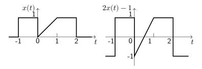
Time and amplitude transformation of a signal
