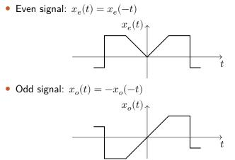
All signals can be represented as the sum of an even signal and an odd signal
